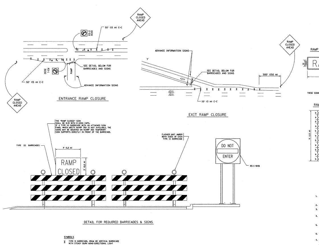
TYPE III BARRICADE WITH FLASHING LIGHT
