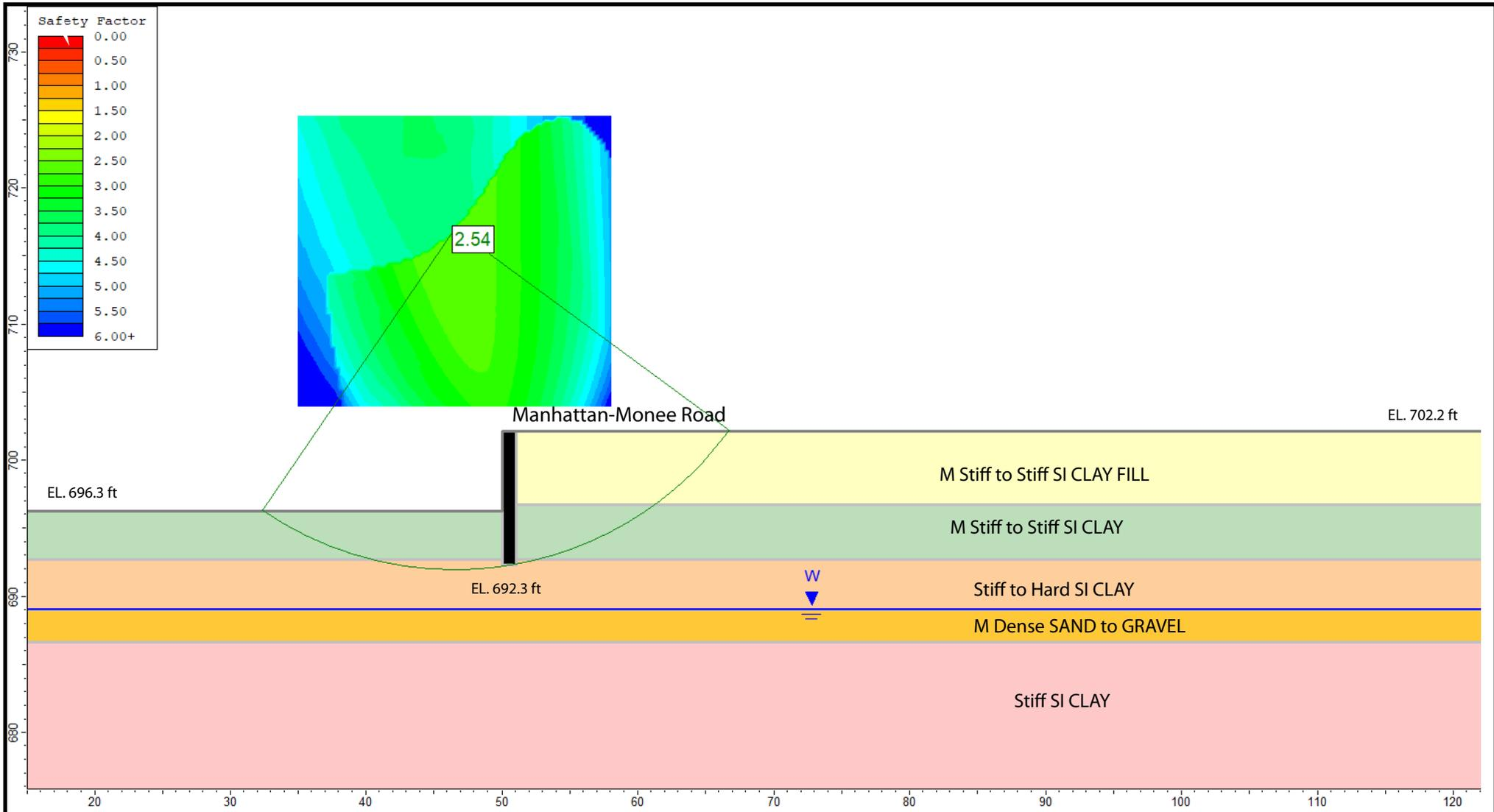
Drained Analysis, Retaining Wall No. 1, Ref Borings: CB-03 and RW-02
