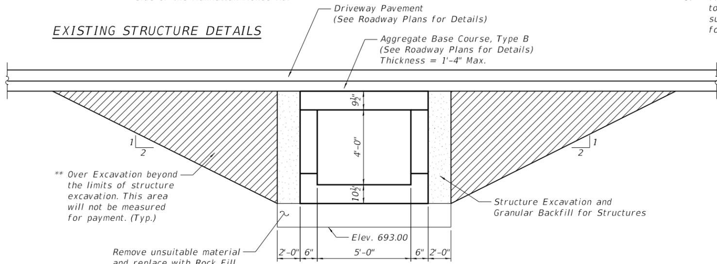
**SECTION THRU CULVERT**
