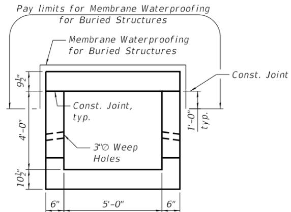
**SECTION THRU CULVERT**
