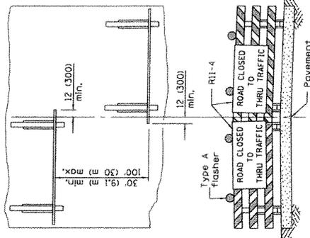
ReflectORIZED striping shall appear on both sides of the barricades. If a Type III barricade with an attached sign panel which meets NCHRP 350 is in use, the signs may be mounted on NCHRP 350 temporary sign supports directly in front of the barricade.
