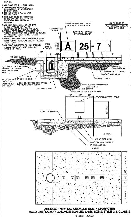
CONTRACTOR SHALL SUBMIT DETAILED SHOP DRAWING INCLUDING SIGN, COLOR, SIZE, PROPOSED LEGEND, IN ENOUGH DETAIL AND DETERMINE NEW SPACING AND OTHER INFORMATION REQUIRED BY SPECIAL PROVISIONS. CONTRACTOR TO VERIFY NEW SIGN LOCATIONS AND ORIENTATIONS WITH RESIDENT ENGINEER PRIOR TO INSTALLATION. SIGN SHALL BE FAA APPROVED LED TYPE SIGN.
