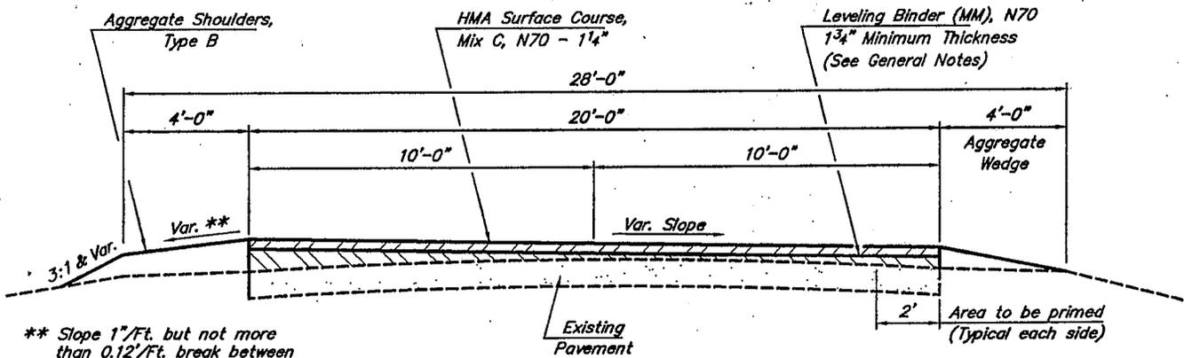
\*\* Slope 1"/ft. but not more than 0.12'/ft. break between pavement and shoulder.
