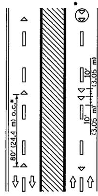
\* Reduce to 40' (12.2 m) o.c. on curves where advisory speeds are 10 mph (15 km/h) lower than posted speeds.
