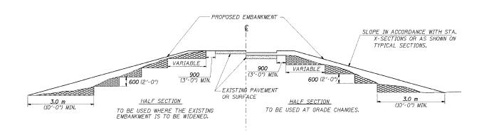
MATERIAL TO BE REMOVED AND REPLACED IN THE EMBANKMENT IN ACCORDANCE WITH ART. 205.04 OF THE STANDARD SPECIFICATION. COST TO BE INCLUDED IN THE VARIOUS ITEMS OF EXCAVATION AND NO ADDITIONAL COMPENSATION WILL BE ALLOWED BECAUSE OF THIS WORK.
