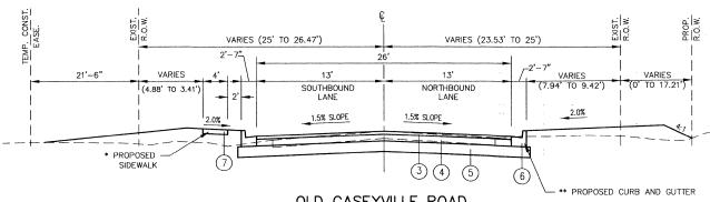
PROPOSED TYPICAL SECTION STA. 12+00.88 TO STA. 14+24.41
