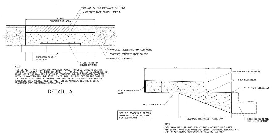
TAPER FROM 2" TO 1-1/2" IN 5 PROPOSED HOT-MIX ASPHALT SURFACE COURSE THICKNESS VARIES (1-1/4" MIN.) -SAW CUT EXISTING HOT-MIX
