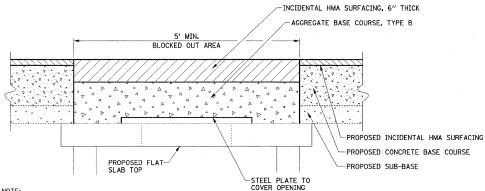
THIS DETAIL IS FOR TEMPORARY PAVEMENT ABOVE PROPOSED STRUCTURES. THE TEMPORARY PAVEMENT IS REQUIRED UNTIL THE PROPOSED CASTING IS ADJUSTED TO GRADE AFTER THE HMA RESURFACING IS COMPLETE AND THE PROPOSED CONCRETE PATCH IS CONSTRUCTED. THE STEEL PLATE SHALL BE INCLUDED IN THE COST OF THE PROPOSED DRAINAGE STRUCTURE. THE INCIDENTAL HMA SURFACING AND THE AGGREGATE BASE COURSE WILL BE PAID FOR SEPARATELY. SEE THE SPECIAL PROVISIONS FOR ADDITIONAL INFORMATION.
