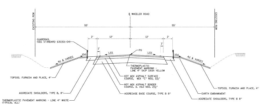
PROPOSED TYPICAL ROADWAY SECTION STATION 14+30 TO STATION 16+67 NOT TO SCALE
