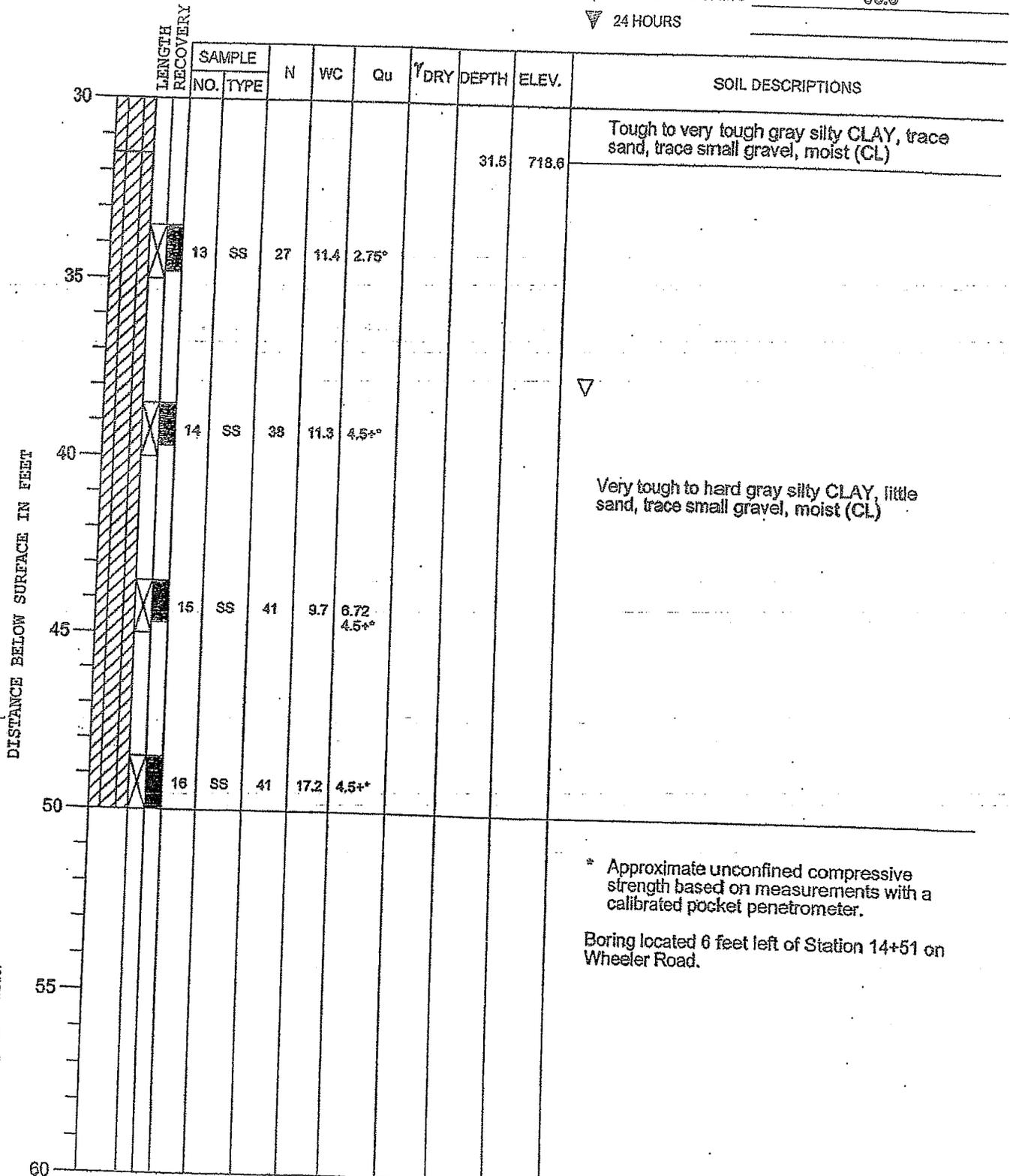
\* Approximate unconfined compressive strength based on measurements with a calibrated pocket penetrometer.
