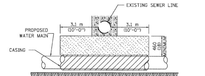
CASING SHALL BE CAST IRON WITH AN INSIDE DIAMETER 50 (2) LARGER IN DIAMETER THAN ENCASED PIPE OUTSIDE DIAMETER WITH BOTH ENDS OF CASING SEALED
