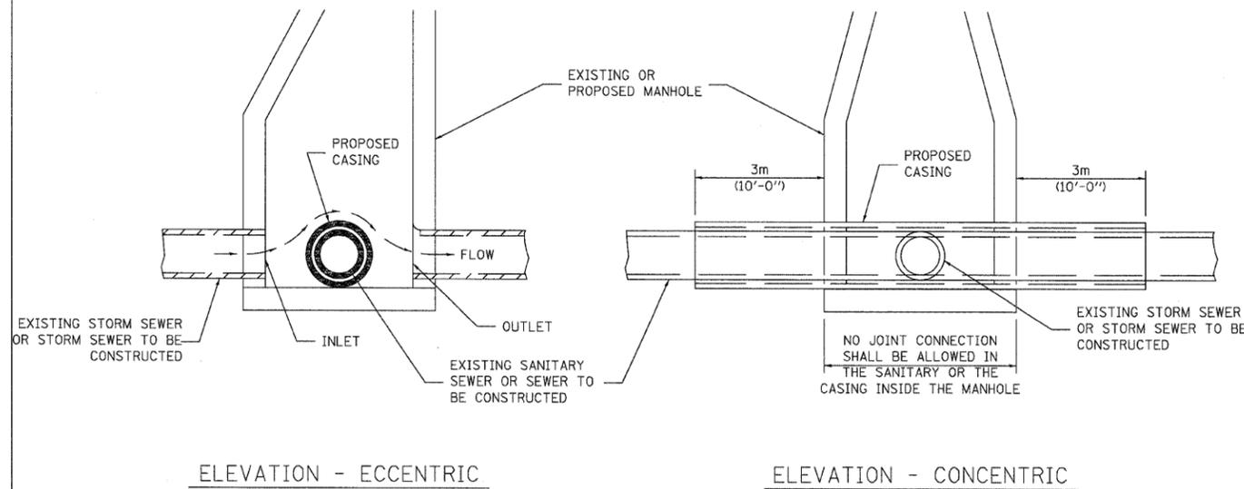
CASING SHALL BE CAST IRON WITH AN INSIDE DIAMETER 50 (2) LARGER IN DIAMETER THAN ENCASED PIPE OUTSIDE DIAMETER WITH BOTH ENDS OF CASING SEALED
