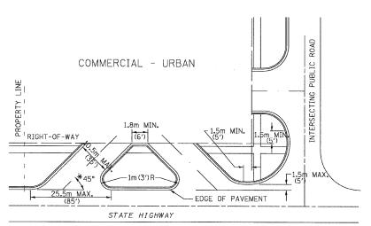
WHEN THE ISLAND BETWEEN DRIVES IS LESS THAN 7.5m (25') LONG OR LESS THAN 10 FEET WIDE, IT SHALL BE DEFINED BY CURBS, MASONRY. OR OTHER DEVICES.
