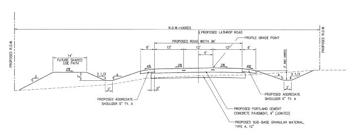
PROPOSED TYPICAL CROSS-SECTION LATHROP STREET STA. 15+00 TO STA. 18+00
