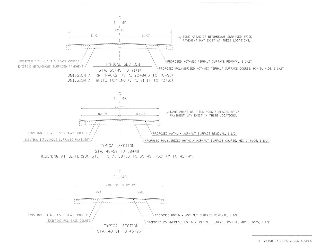
DESIGNED REVISED DRAWN REVISED STATE OF ILLINOIS TYPICAL SECTIONS 72\_sht\_pln.dqn UNION 24 6 **DEPARTMENT OF TRANSPORTATION** LOT SCALE = 5.0000 '/ IN. CHECKED REVISED CONTRACT NO. 78072 SHEET NO. OF SHEETS STA. SCALE: TO STA.
