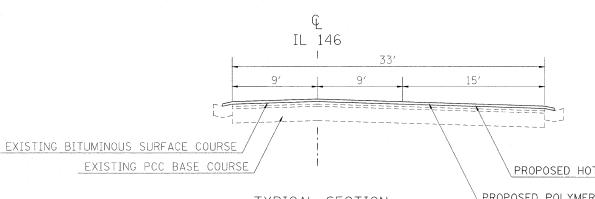
PROPOSED HOT-MIX ASPHALT SURFACE REMOVAL, 1 1/2"
