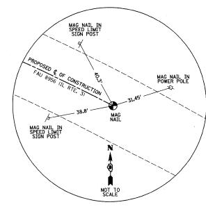
P.T. STA. 646+22.35 PROPOSED ¢ OF CONSTRUCTION FAU ROUTE 8956 / IL RT. 3 SET MAGNAIL
