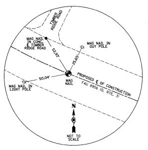
P.T. STA. 631+77.44 PROPOSED ¢ OF CONSTRUCTION FAU ROUTE 8956 / IL RT. 3 SET MAGNAIL
