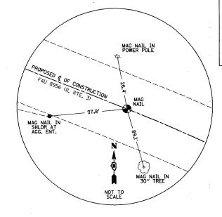
P.C. STA. 642+97.06 PROPOSED ¢ OF CONSTRUCTION FAU ROUTE 8956 / IL RT. 3 SET MAGNAIL
