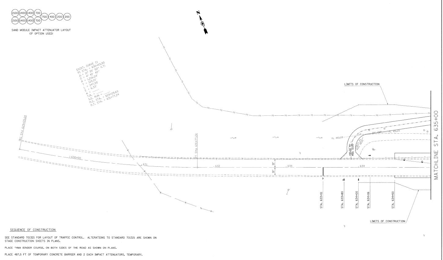
REMOVE SKIP-DASH AND SOLID EDGE PAVEMENT MARKING BETWEN STOP BARS.
