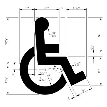
TYPICAL DETAIL FOR PAINTING HANDICAP MARKINGS
