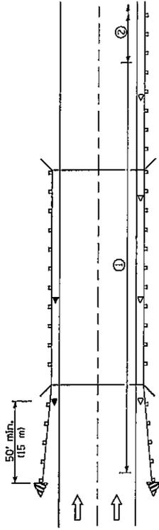
① Spacing 80 ft. (24 m) max. for first 400 ft. (122 m) or curve spacing shown in Standard 635001, whichever is less (min. 4 reflectors regardless of length).
