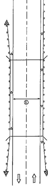
③ Bidirectional silver/silver should be used in lieu of monodirectional silver on both sides of two-lane bridges where the pavement is less than 24 (7.6) wide than the pavement approaching the bridge.
