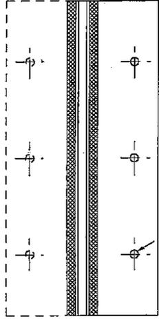
3 min. adhesive weep holes or slots each side, variable spacing.
