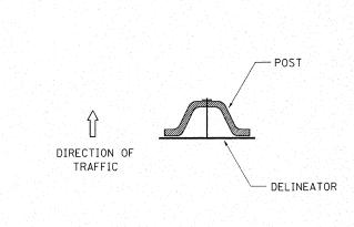
DELINEATORS SHALL BE INSTALLED ACCORDING TO STANDARD 635001 EXCEPT THAT THE POST SHALL BE ROTATED 180°. THE POST WILL HAVE THE WIDE SIDE FACING TRAFFIC AND THE DELINEATOR ATTACHECD AS SHOWN ABOVE.
