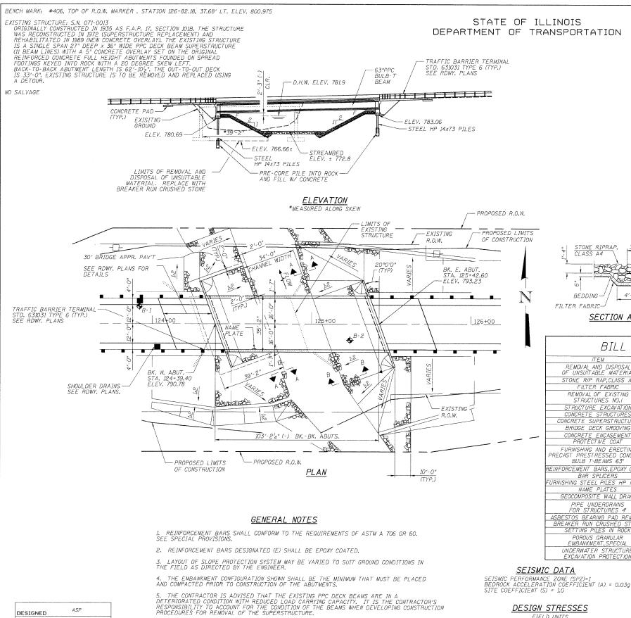
6. ALL EMBEDDED AND SEPARATE BEARING PLATES, SIDE RETAINERS, ANCHOR BOLTS, NUTS, WASHERS, AND PINTLES SHALL BE GALVANIZED ACCORDING TO AASHTO M111 OR M232 (AS APPLICABLE).
