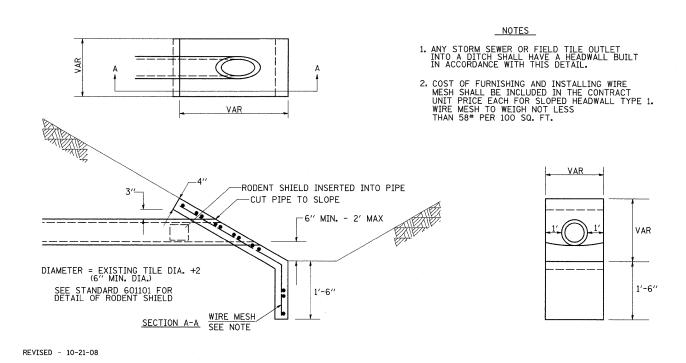
SLOPED HEADWALL TYPE 1 FOR FIELD TILE OUTLETS
