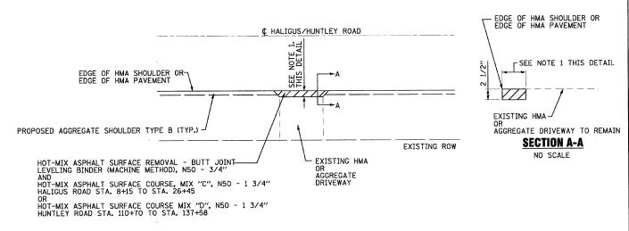
NOTE: 1. 5' MIN. WHEN MATCHING EXISTING HMA DRIVEWAY UNLESS OTHERWISE DIMENSIONED 3' MIN. WHEN MATCHING EXISTING AGGREGATE DRIVEWAY UNLESS OTHERWISE DIMENSIONED
