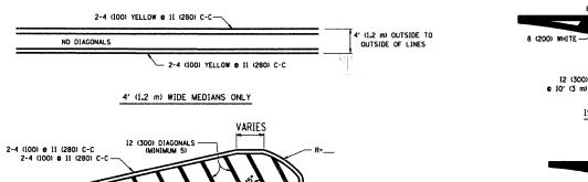
FOR MEDIAN LENGTHS WHERE DIAGONAL SPACING CANNOT BE ATTAINED, USE 5 (FIVE) EQUALLY SPACED DIAGONAL LINES.
