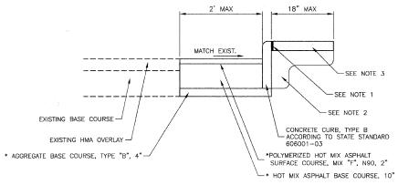
**CURB & GUTTER REMOVAL DETAIL**
