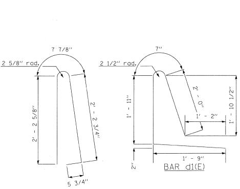
Parapet Reinforcement Detail
