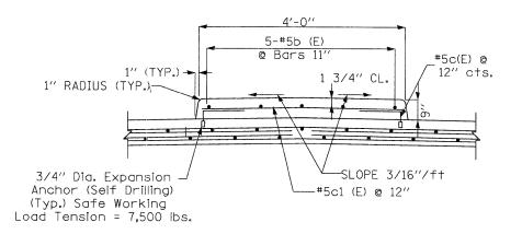
CONCRETE MEDIAN AT APPROACH SLABS
