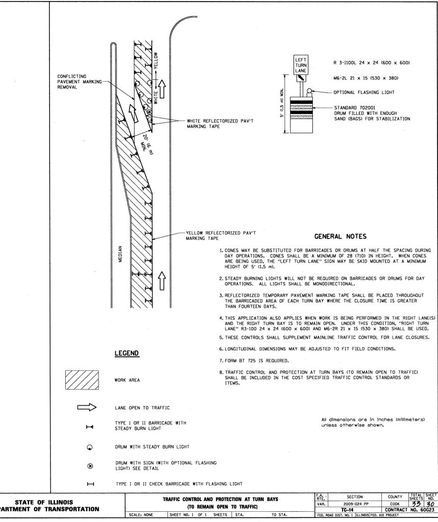
REVISED -T. RAMMACHER 09-08-94 FILE NAME = DESIGNED USER NAME = smithkl c:\pw\_work\PWIDOT\SMITHKL\dØ125Ø91\Dis DRAWN REVISED - A. HOUSEH 11-07-95 CHECKED PLOT SCALE = 100.0000 '/ IN. REVISED - A. HOUSEH 10-12-96 DATE REVISED -T. RAMMACHER 01-06-0 PLOT DATE = 2/3/2009
