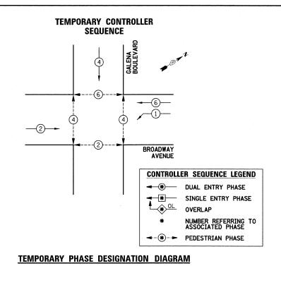
PUSHBUTTONS "A" SHALL PLACE A CALL IN PHASES 2 AND 4
