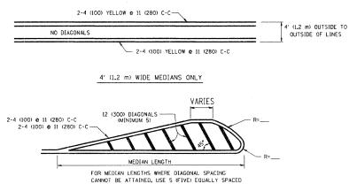
DIAGONAL LINE SPACING: 50' (15 m) C-C (LESS THAN 30MPH (50 km/h)) 75' (25 m) C-C 30MPH (50 km/h) TO 45MPH (70 km/h)) 150' (45 m) C-C (MORE THAN 45MPH (70 km/h))
