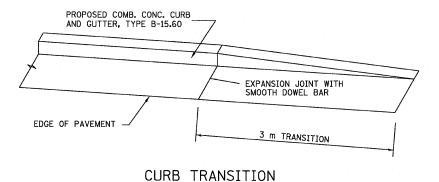
NOTE: TRANSITION CURB SHALL BE PAID FOR AS COMB. CONC. CURB & GUTTER, TYPE B-15.60
