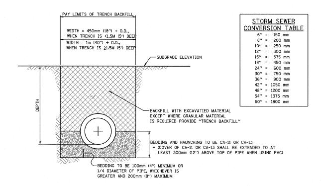
NOTES: TRENCH WIDTH SHALL BE AS NARROW AS POSSIBLE, WITH MINIMUM WIDTH OF PIPE O.D. PLUS 200mm (8") ON EACH SIDE.
