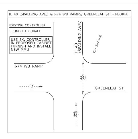
THE CONTRACTOR SHALL FURNISH AND INSTALL A MALFUNCTION MANAGEMENT UNIT (RENO 1600MM2) WITH EACH CONTROLLER CABINET. THE COST OF THE MALFUNCTION MANAGEMENT UNIT SHALL BE INCLUDED IN THE COST OF THE PROPOSED TRAFFIC SIGNAL CABINET.
