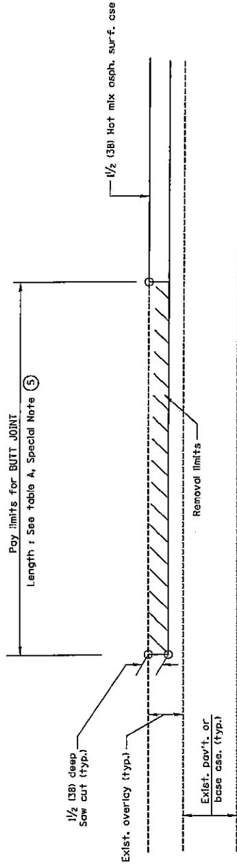
CASE 5 : WITH HOT MIX ASPHALT SURFACE REMOVAL (COLD MILLING)
