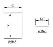
EXPANSION BOLTS SHALL CONSIST OF SELF DRILLING EXPANSION SHIELDS AND 3/4 " DIA. HOOKED BOLTS. HOOKED BOLTS SHALL EXTEND A MINIMUM OF 9" INTO NEW CONCRETE. BOLTS SHALL BE DRILLED IN THE CENTER OF THE EXISTING BOX CULVERT BARREL WALLS.
