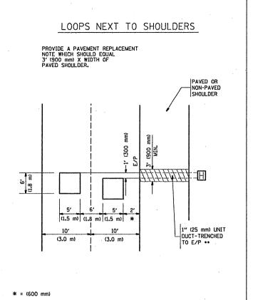
\* \* LINIT DUCT IS TO BE SHOWN ON PLAN SHEETS
