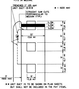
NOTE: DUAL LEFT TURNS NOT SHOWN REFER TO PLAN SHEET FOR DETECTOR LOOP REPLACEMENT
