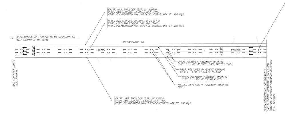
APPROACH ROADWAY RESURFACING TO BE PERFORMED AT NORTH AND SOUTH APPROACHES OF S.N. 016-2407.
