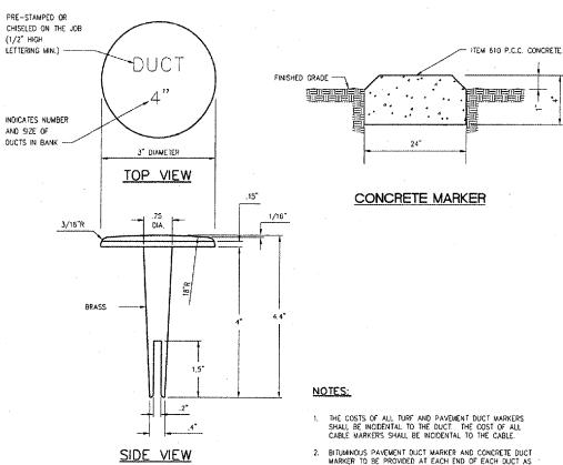
NOTE: TOP OF MARKER SHALL BE FLUSH WITH FINISHED PAVEMENT SURFACE. MARKER MAY BE INSTALLED IN A DRILLED HOLE AND SECURED WITH EPOXY GLUE.
