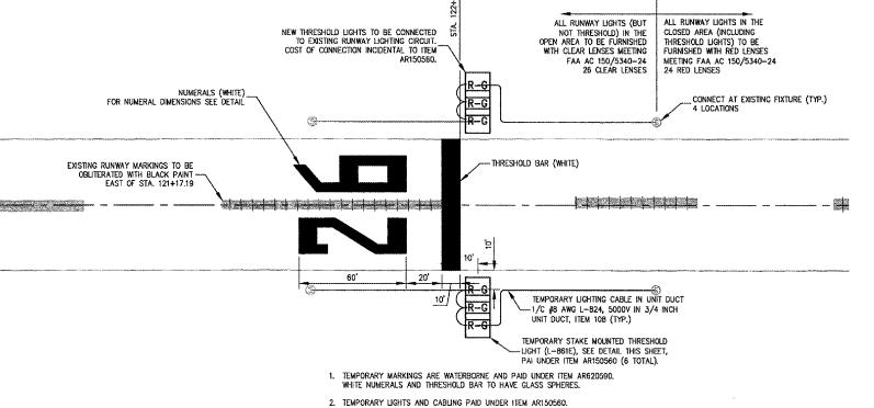
**TEMPORARY** THRESHOLD MARKINGS AND LIGHTING DETAIL
