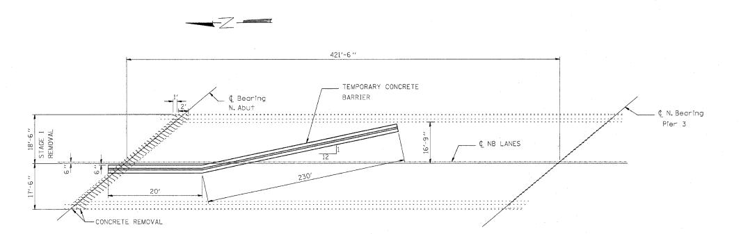
TYPICAL PLACEMENT OF TEMPORARY CONCRETE BARRIER
