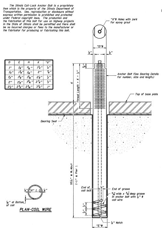
ILLINOIS COIL-LOCK ANCHOR BOLT
