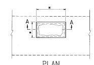
\* LIMITS OF PARTIAL DEPTH PATCHING AS DIRECTED BY THE ENGINEER,
