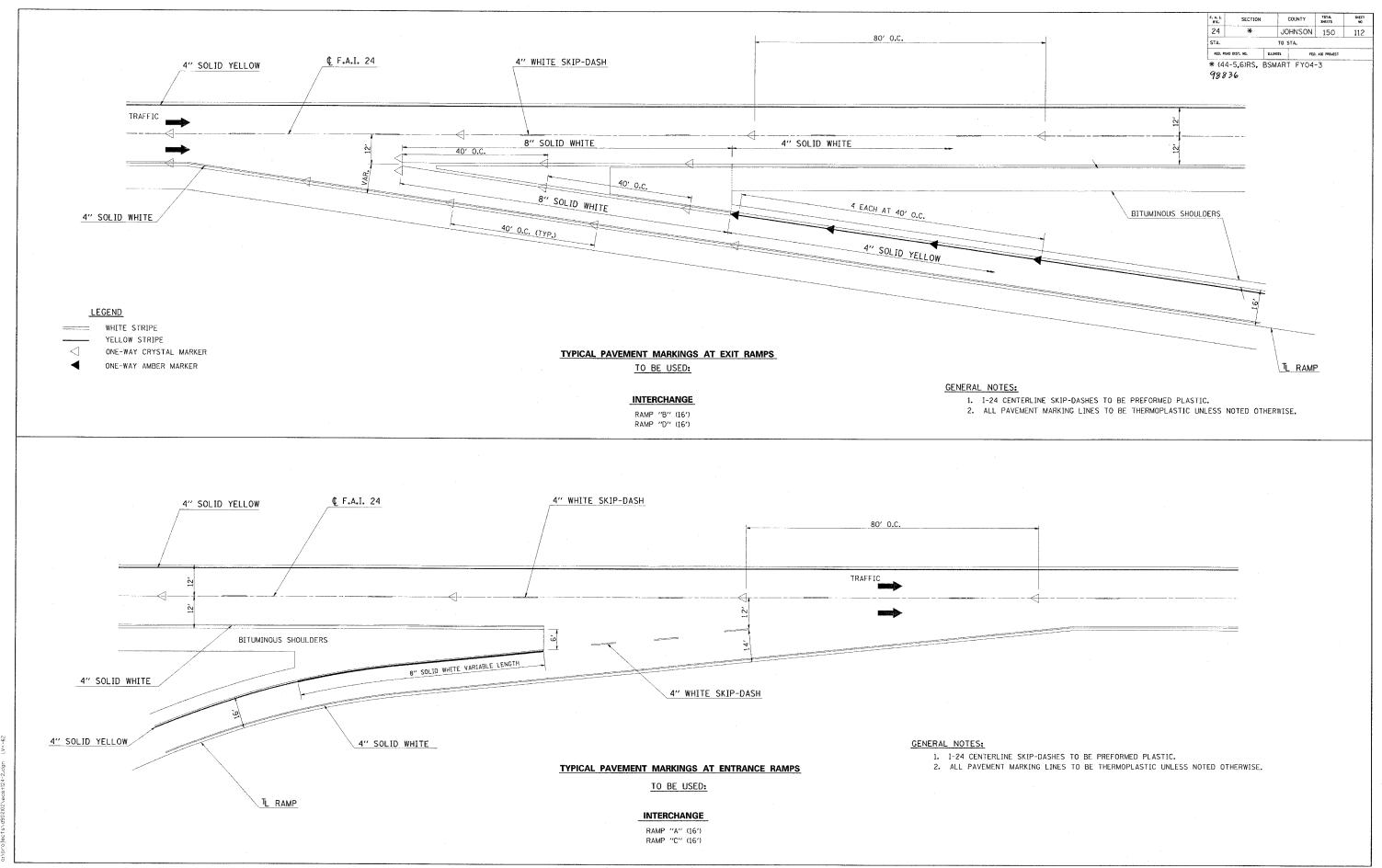
DETAILS - TYPICAL PAVEMENT MARKINGS AT ENTRANCE RAMPS;
