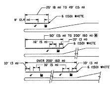
\* TURN LAMES IN EXCESS OF 400' (120 m) IN LENGTH MAY HAVE AN ADDITIONAL SET OF ARROW - "ONLY" INSTALLED MIDWAY BETWEEN THE OTHER TWO SETS OF ARROW - "ONLY".
