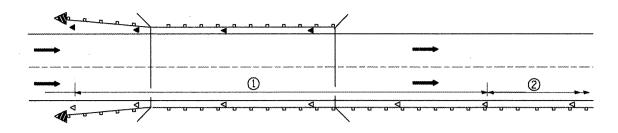
① Spacing 80 ft. (24 m) max. for first 400 ft. (122 m) or curve spacing shown in Standard 635001, whichever is less (min. 4 reflectors regardless of length).
