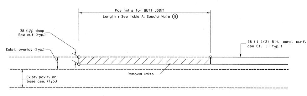
CASE 5: WITH BITUMINOUS SURFACE REMOVAL (COLD MILLING)
