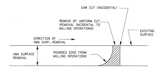
NOTE: WHEN MILLING OPERATIONS PRODUCE A ROUNDED EDGE,
