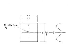
Plate A shall be placed between rall element and block-out at non-splice mounting points only when steel block-outs are used.
